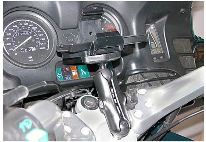
R-A-M Mount in place
